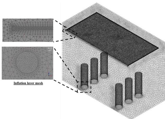
Fig.2 Grid of the simulation domain and the inflation layers
