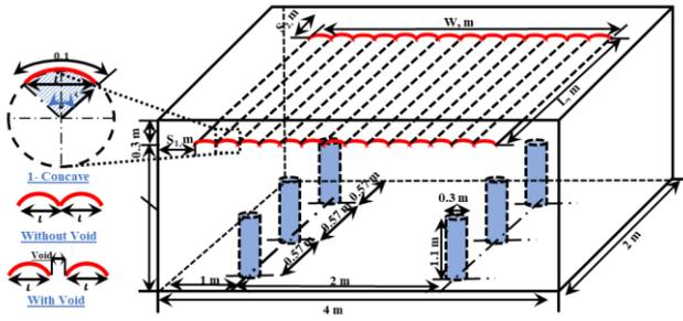
Fig. 1 Geometric dimensions used in this study
