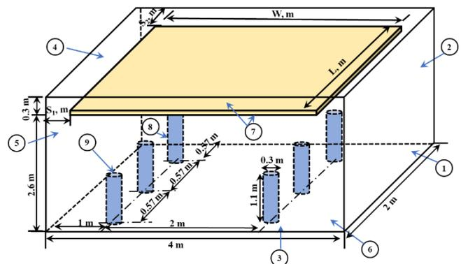
Fig. 3 Boundary conditions used in this study
