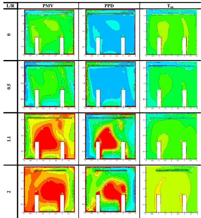
Fig. 10 PMV index, PPD index and Operative temperature.
